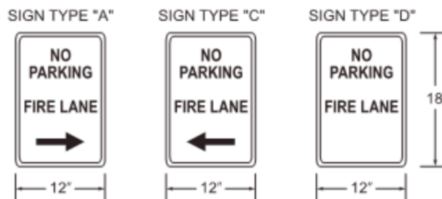
FIGURE D103.6 FIRE LANE SIGNS
